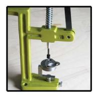
The Unilock Press can be screwed half-way out from the edge of the bench in order to accommodate bangles and other large rounded forms that can rest with their top part over the jig base and the lower part hanging under the press. Jig base supports are needed for this operation.
